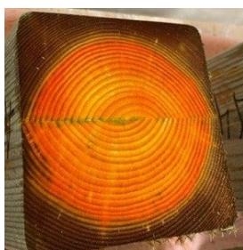
Figure 2. a Duolam with with heartwood glued face to face. b Glulam with three laminations successfully treated after assembling.
