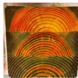
Figure 2. a Duolam with with heartwood glued face to face. b Glulam with three laminations successfully treated after assembling.
