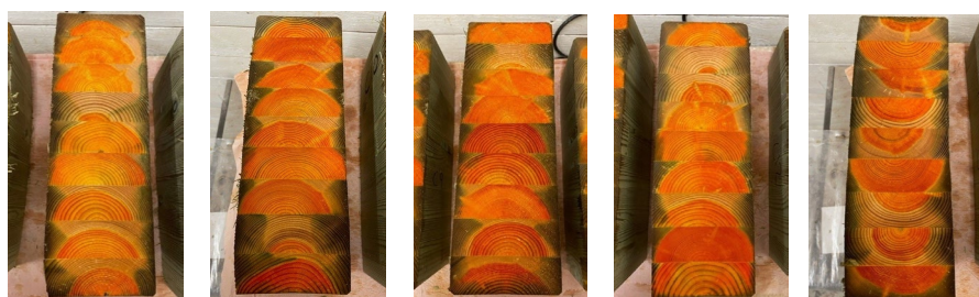
Figure 1. Difficulties to comply with NTR A and NTR AB penetration requirement of full sapwood when treating after assembling.
